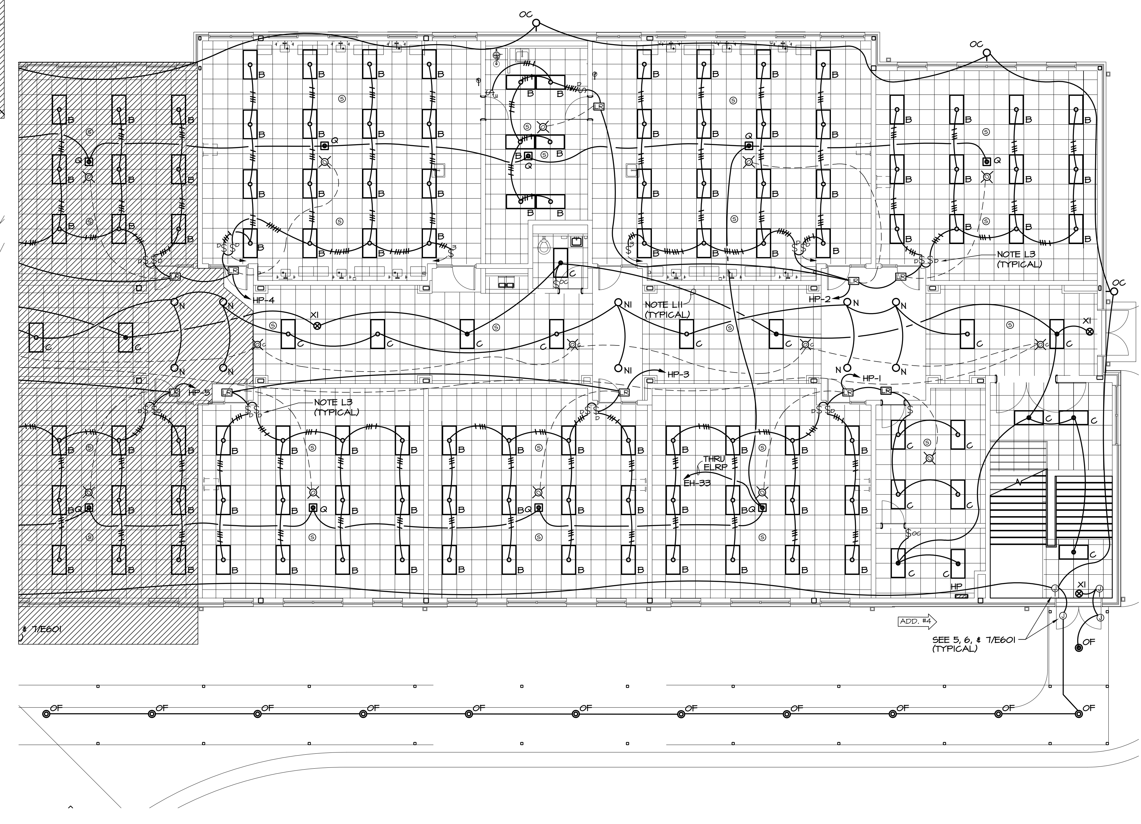
2 PARTIAL LOWER LEVEL FLOOR PLAN - LIGHTING E10 1/8"=1'-0"
